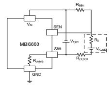
Figure 3. The equivalent impedance of MBI6661 application circuit
