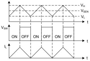
Figure 2 Waveforms of hysteretic PFM control scheme
