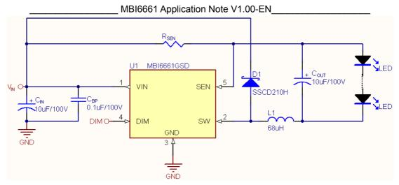
Figure 1 Application circuit of MBI6661
