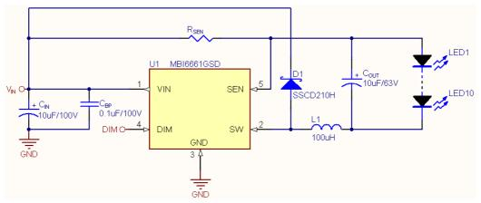
Figure 4. The application circuit of design example
